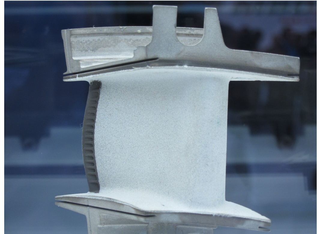
Ceramic thermal barrier coating (TBC) on turbine guide vane.
